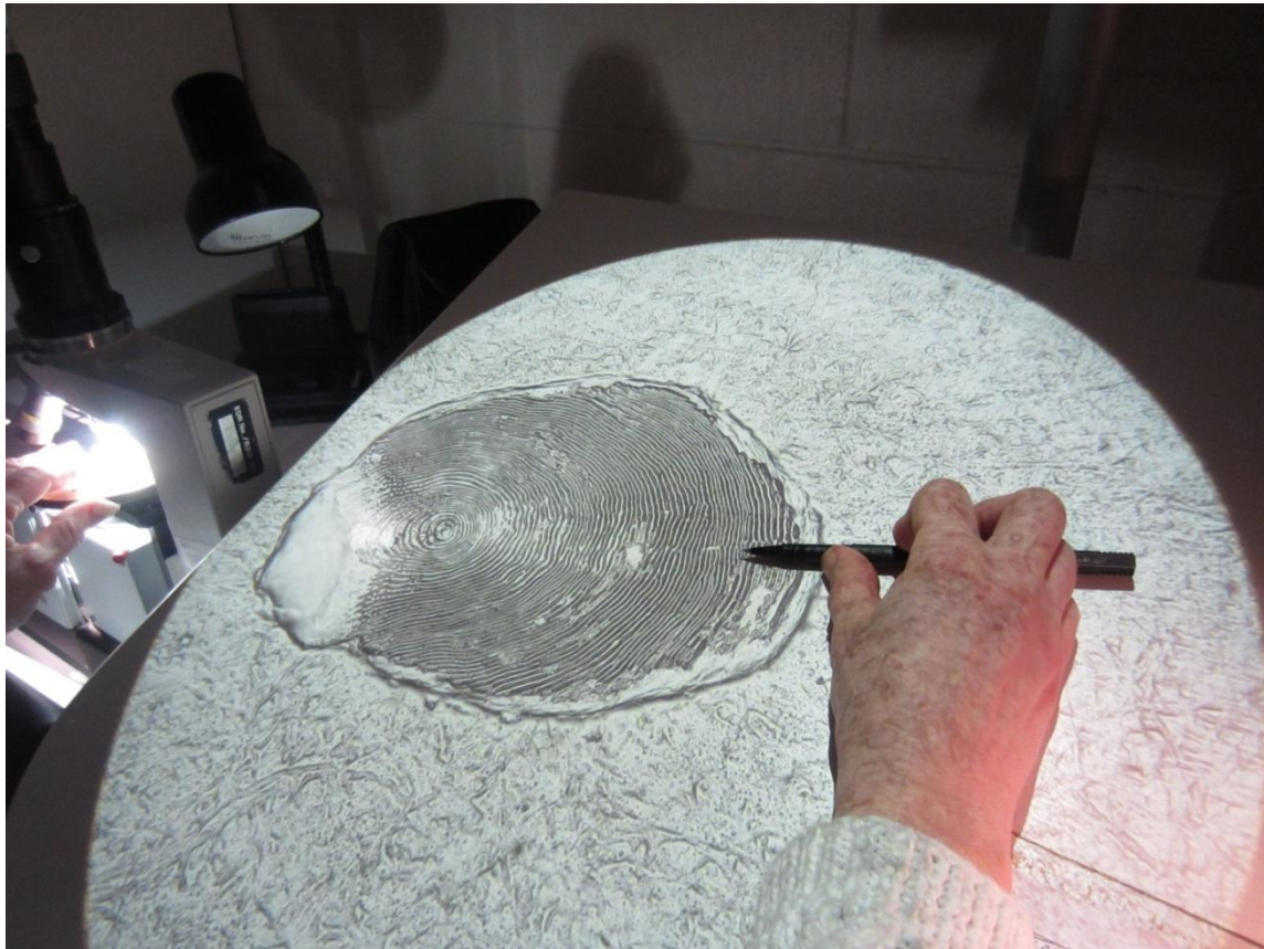
Fig. 12 Photo demonstrating how SCL salmon readers use a pen to “measure” the size of annual growth zones on the scale image.
